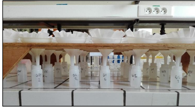
Figure 11: Extraction of bioavailable silicon extracted with \text{CaCl}_2
