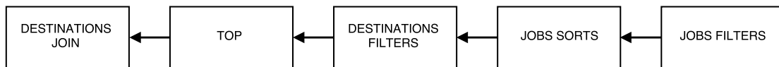
Fig. 4.2 Simplified query execution plan generated for a query on Jobs and Destinations tables, linked by a join.
