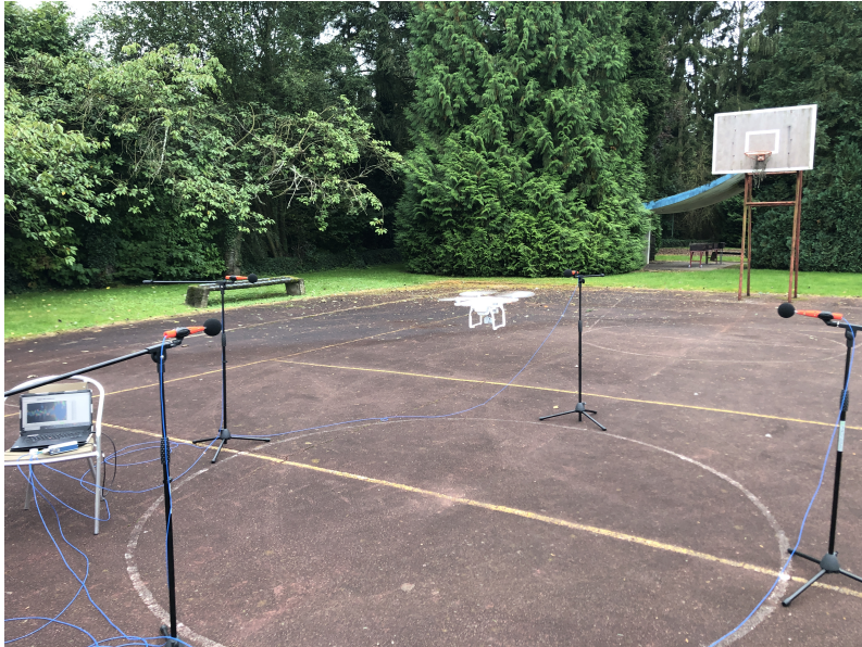
FIGURE 3.7: Outdoor experiments on the von Karman Institute's campus. The microphones are in a square configuration and connected to the acquisition system and to Lab-View on the PC.
