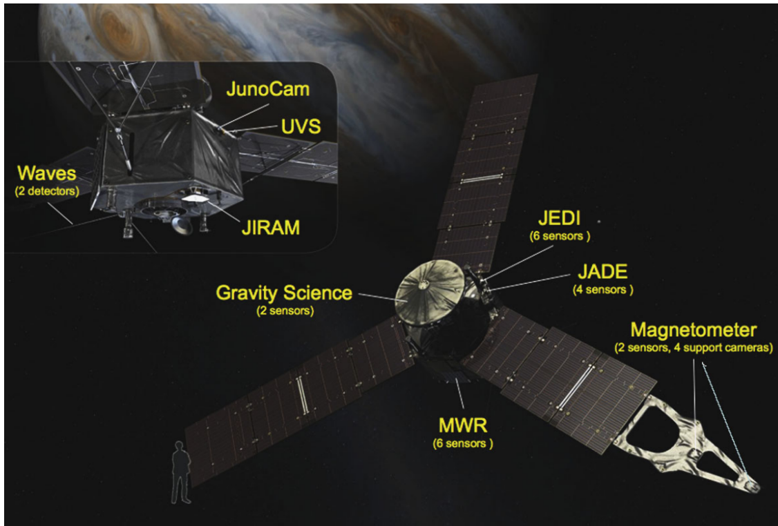
Figure 2.3: The Juno spacecraft. All the scientific instruments onboard are labelled. From [Bolton et al., 2017].
