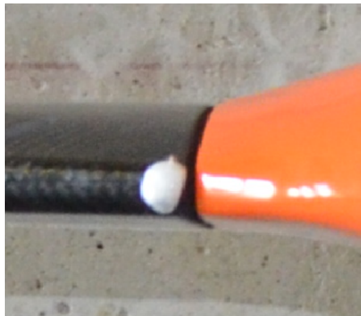
Figure 3.9: Direct contact between the wing and the fuselage on the prototype UAV
