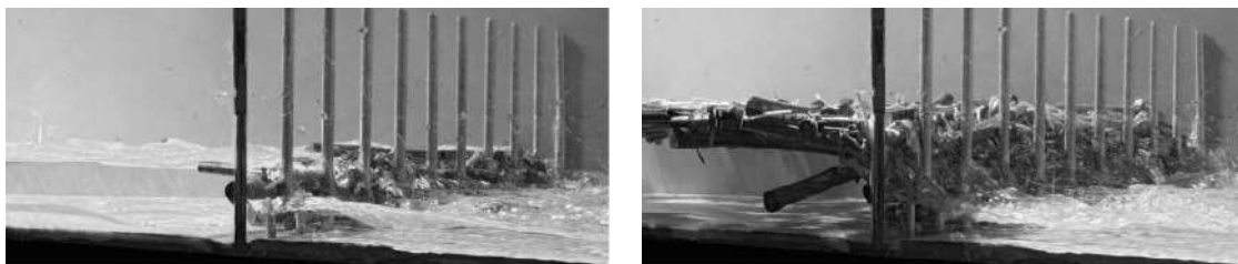
(a) Schmocker and Hager, 2013, fig.3, Initial debris accumulation.
