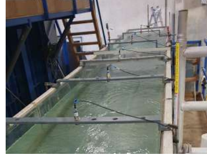
Figure 16: Sensors in the flume.
