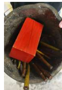
Figure 37: Volume of debris that passed the bridge after the launch of the first batch during the test C51\_1p ( h_0 = 200mm , Fr_0 = 0.4 )
