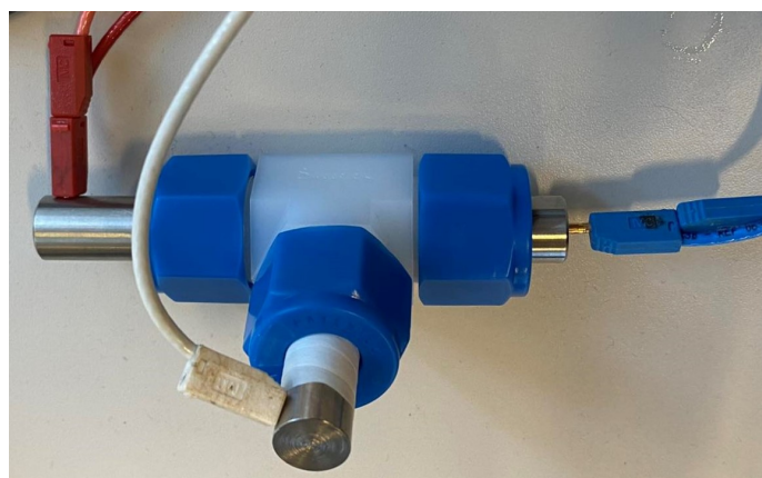
Figure 2.18: Assembled Swagelok T-cell connected to the VMP3 Biologic potentiostat.
