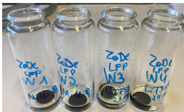
Figure 2.12: Set-up for the electrode stability test in the water-in-salt electrolyte.
