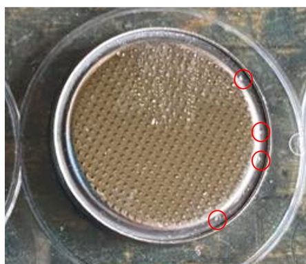
Figure 4.8: Drops formed on the seal of the coin cells during cycling. The drops are indicated by the red circles.
