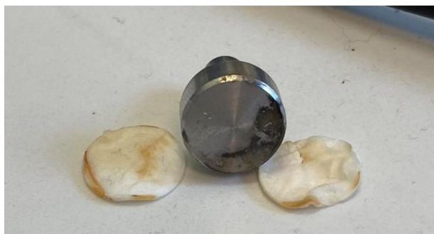
Figure 2.25: State of the separators and the working electrode after the cyclic voltammetry measurements of the water-in-salt electrolyte in three-electrode system.
