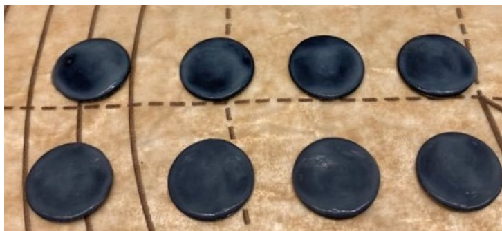
Figure 3.2: GPE casted on the LFP (first row) and LTO (second row) electrodes by drop-casting.
