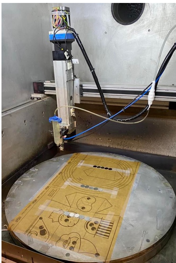
Figure 1.5: Set-up for the spray-coating process.
