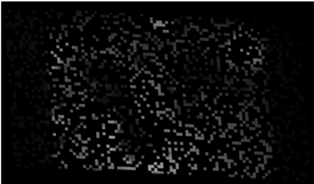
Figure 53: Laboratory image masked with a CS ratio of 25% and a binning of 20 by 20 on the DMD.
