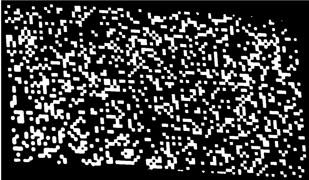
Figure 52: Mask with a CS ratio of 25% and a 20 \times 20 binning on the DMD.
