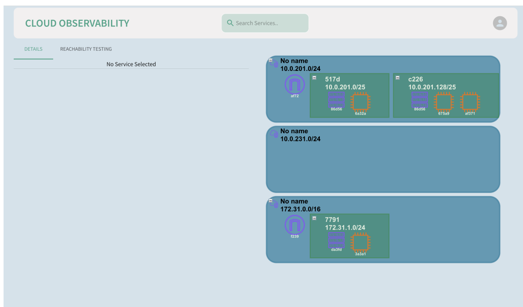
Figure A.3: Main page showcasing your infrastructure on the right, with visible details of three VPCs, including their CIDR range and name (if tagged). Subnets are shown along with their CIDR range and last digits of their ID (with an option to display their name). The left pane contains two tabs, for viewing clicked service details and performing reachability testing.
