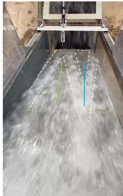
FIGURE 4.22: Flow downstream PKW2.
