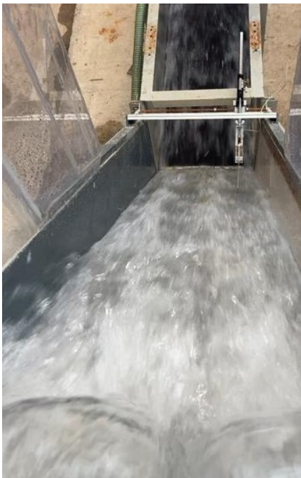
FIGURE 4.1: Flow downstream PKW1.
