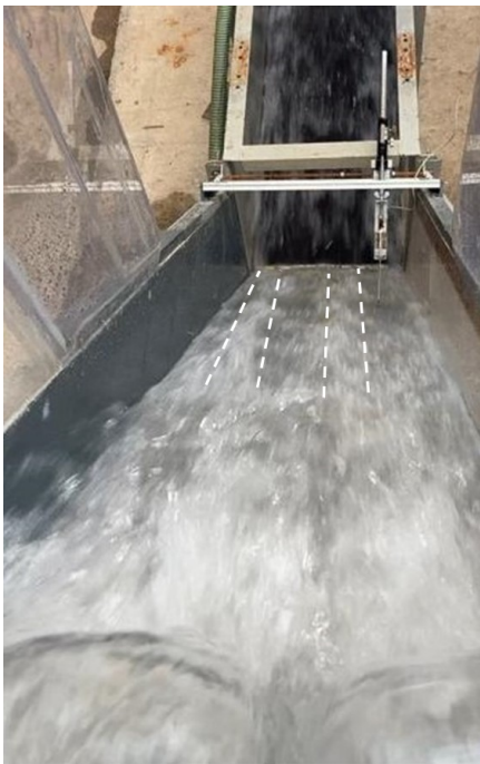
FIGURE 4.21: Flow downstream PKW1.
