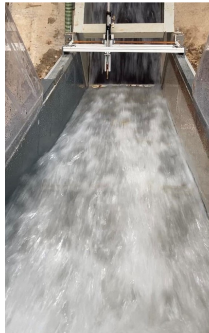
FIGURE 4.2: Flow downstream PKW2.
