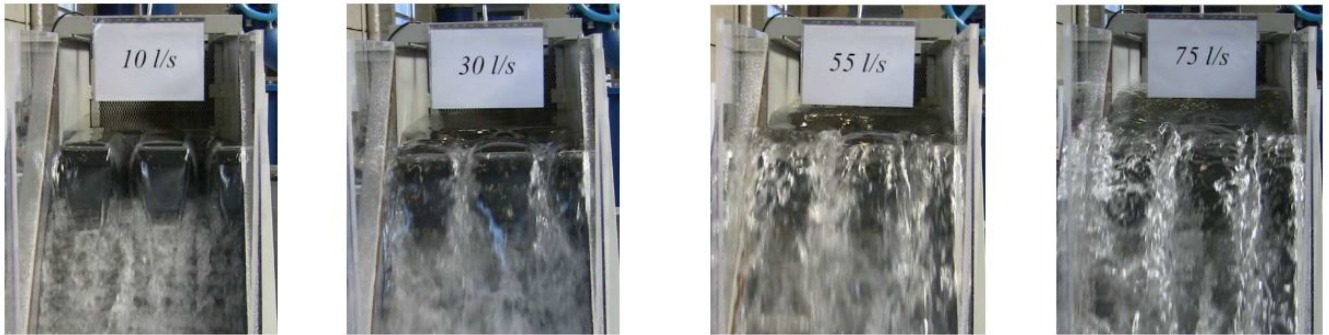
FIGURE 2.13: Nappes interactions depending on the discharge (Silvestri, 2011-2012).
