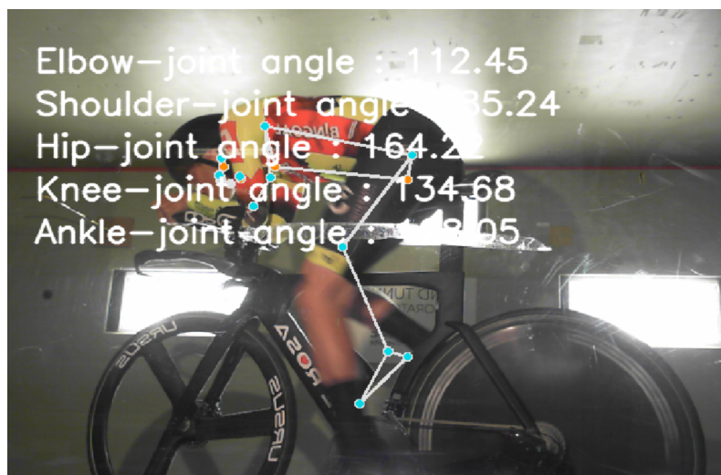
Figure 5.9: Detection of the position of the cyclist using Mediapipe Pose algorithm for the cyclist in the wind tunnel.
