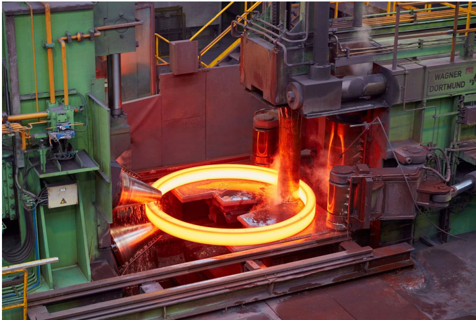
Figure 55: Production rolling forging equipment to manufacture rings and collars [9].
