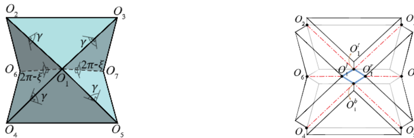
Figure 3.7: Left side shows the model with thin panels, right side shows the one with thick panels [37].
