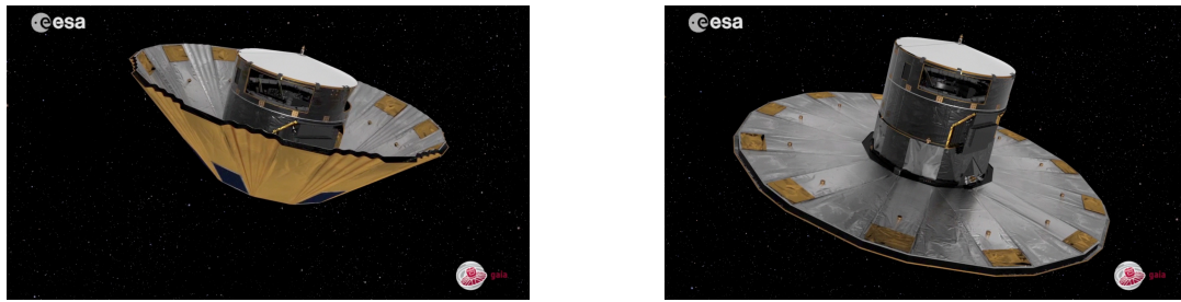
Figure 3.3: Left side shows GAIA's sunshield during its deployment, right side shows GAIA's sunshield fully deployed [34].
