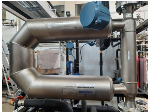
Figure 3.6: The installed CMF200 Coriolis flow and density meter of Emerson Micromotion Elite series.
