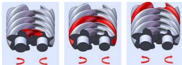
Figure 2.3: Working principle of a twin screw expander. (source :[21])
