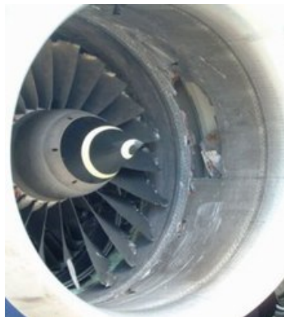
Figure 1.2: Damaged engine fan case from blade-off testing [39].
