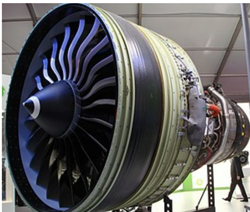
Figure 2.2: Engine GE90-115B soft-wall fan containment system [6]. It is composed by an inner metallic ring wrapped in Kevlar layers.
