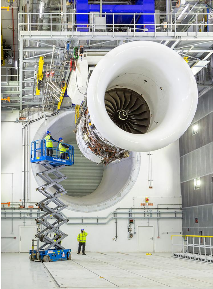
Figure 1.4: Rolls Royce Test Rig installation for the UltraFan [44].
