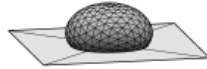
(c) Shape of the droplet with \theta = 135^\circ and g = 5 in dimensionless unit.
