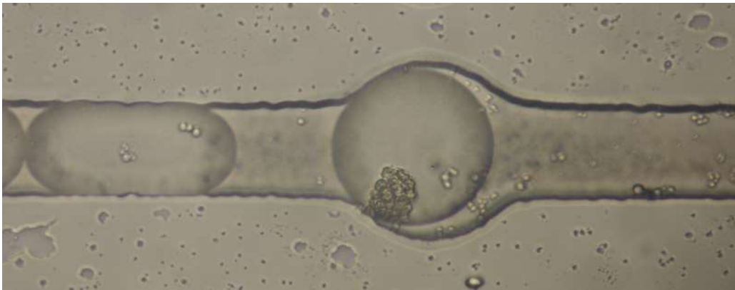
Figure 10.9: Experimental picture showing the formation of a spheroid within the droplet chip. The height is set at H = 80 [ \mu\text{m} ]. The approximate volume of the droplet is estimated to be 1000 [pL].
