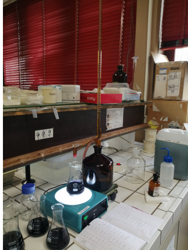
Figure 14: Titration of dichromate potassium excess by Mohr's salt.
