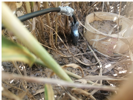
Figure 15: 5TM sensor introduced next to a white collar.
