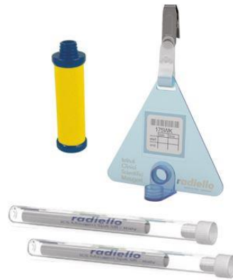
Figure 2. Radiello® sampling material (“Radiello passive samplers. | Markes International,” n.d.)
