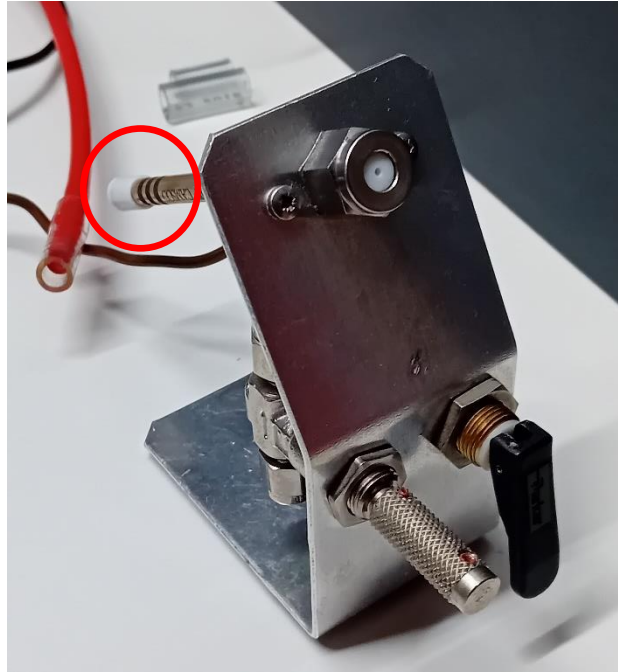
Figure 8. Thermal desorption cartridge containing a Radiello® tube fixed onto the loading rig - note the white cap on the end of the tube
