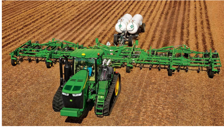
Figure 5: Ammonia Nurse Tanks application as a fertilizer distributor[56]
