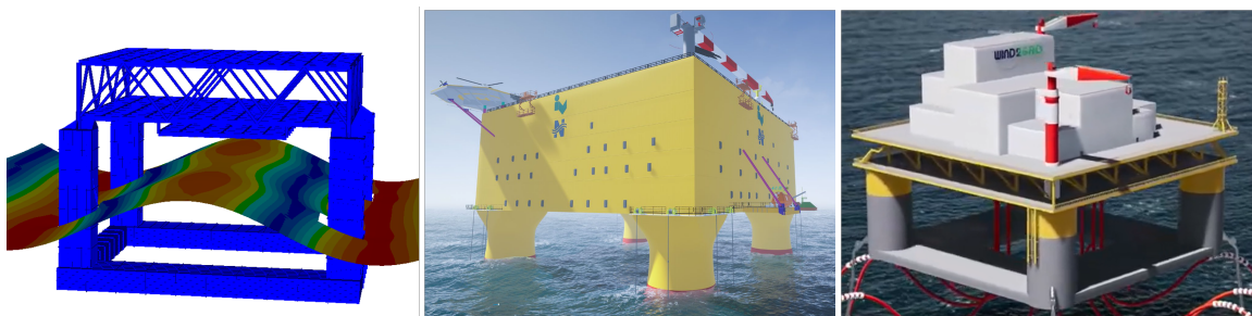
Figure 11. Floating substation concepts, left to right: Linxon (Linxon n.d.), Nevesbu (Nevesbu n.d.), WIND2GRID (WIND2GRID n.d.).
