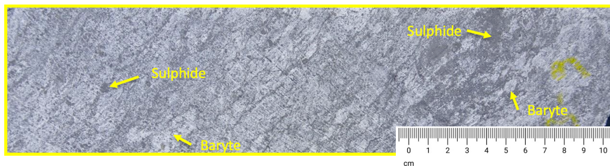
Figure 17. . MACROPHOTO: Ore type 1 – massive barite with minor sulphide (Gn+Sph+Sulph.+Py+Cpy)
