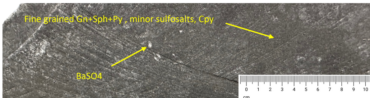
Figure 18. MACROPHOTO: Ore type 2 – massive sulphide (Gn+Sph+Sulf.+Py+Cpy) with minor barite
