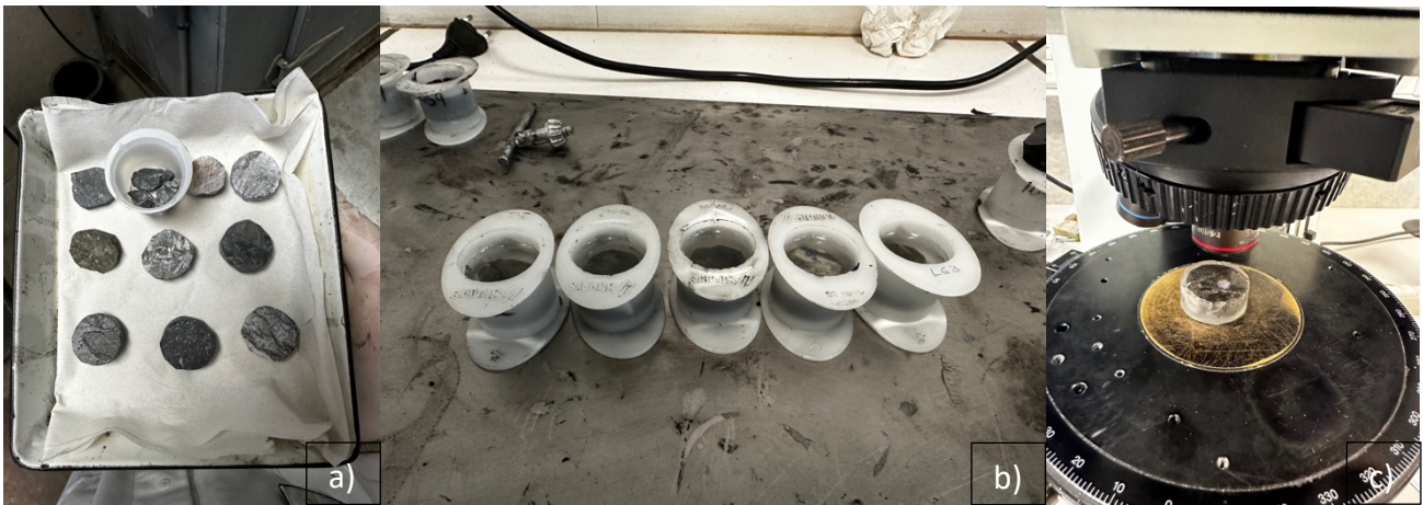
Figure 13. Three step sample preparation for optical microscopy and SEM-EDS. A) core quarters cut in 3cm diameter round shapes, b) EPOFIX resin and moulds in which the samples were put, c) optical microscopy of the samples, checking if the cutting was done properly
