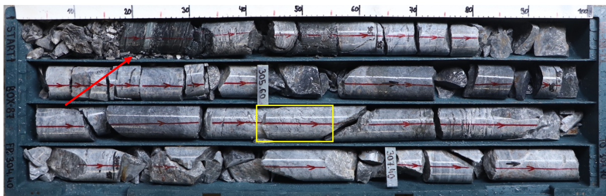
Figure 16. MACROPHOTO: Drillhole BR-08-22, with a clearly visible contact between the fault zone and the massive mineralisation (RED ARROW)
