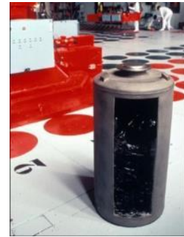
Figure 10: Stainless steel container of vitrified HLW. [ANDRA, 2009c]
