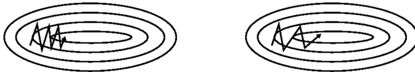
Figure 5.12: Example of the training process without momentum (left) and with momentum (right).
