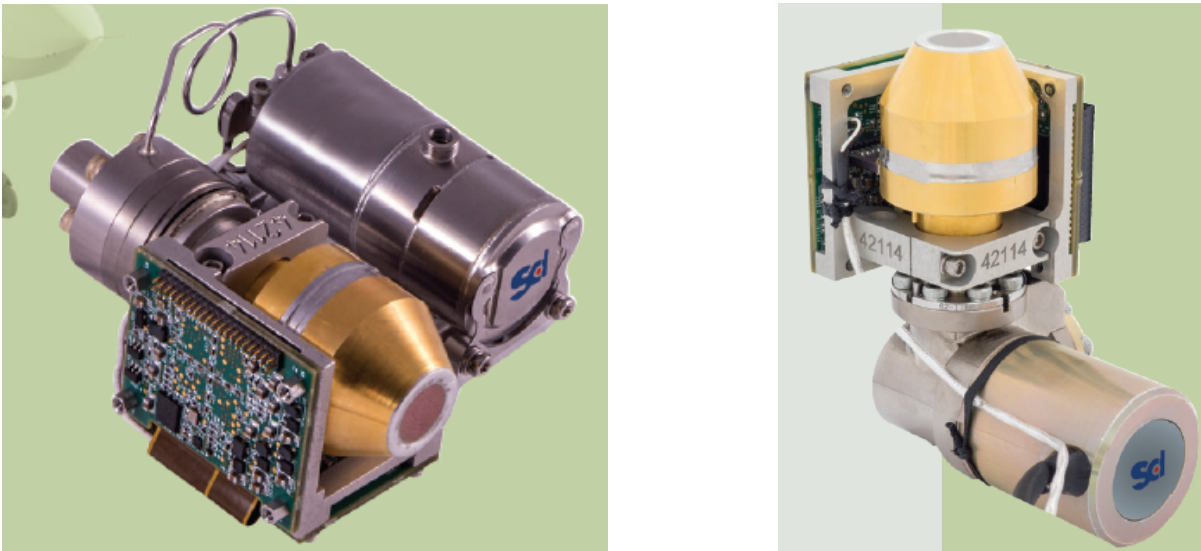
FIGURE 3.4: Kinglet MWIR detector in two configurations
