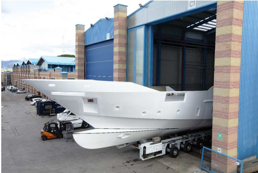
Fig.2.10. The author had edited the copy of the original picture in order to show the featured outline of the blade bow.
