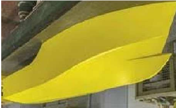
Fig.2.4. Low-scale testing model for towing tank. [8][13]
