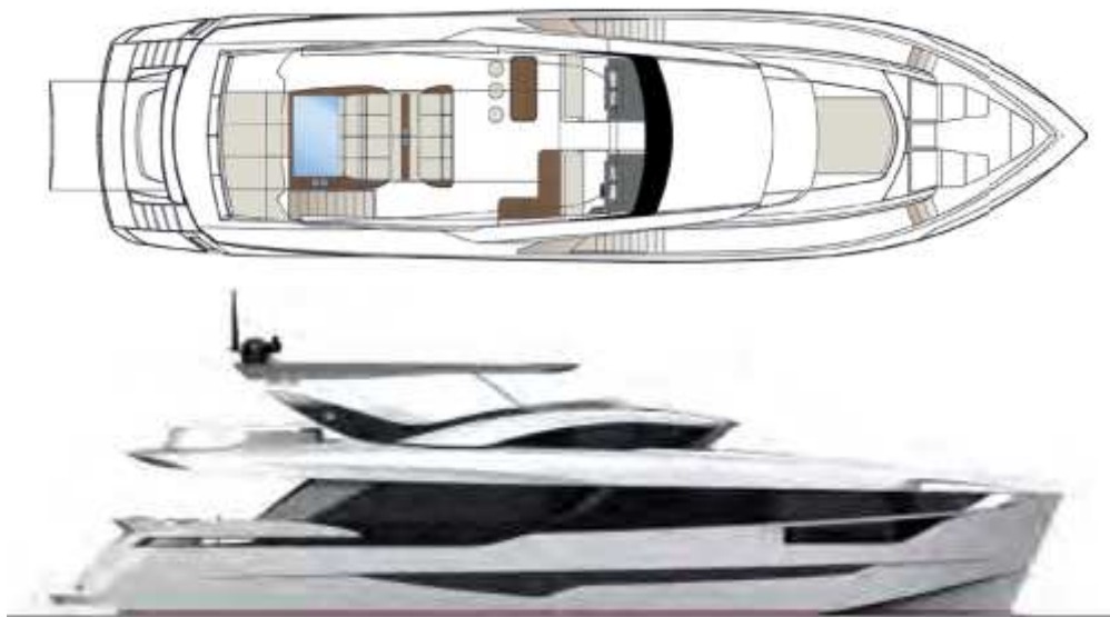
Fig.2.3. The length overall of the Ilumen 28M yacht is 28 meters . The draught of the ship is 1.85 meters (pictures from [5])
