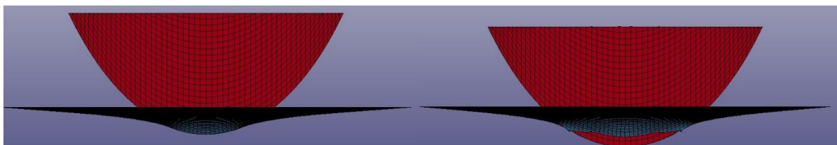
Figure 31 - Total Penetration and Rupture Penetration
