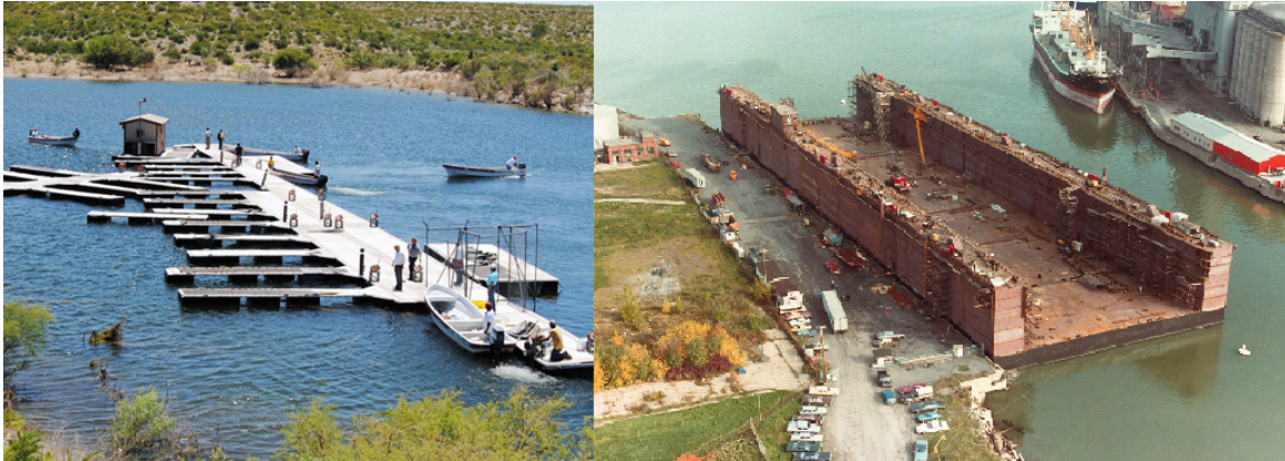
Figure 1: Basic floating dock & Submersible floating dock
