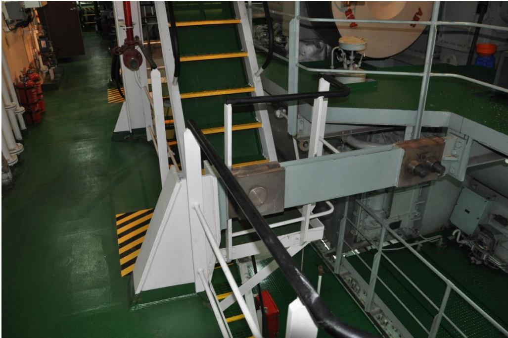
Figure A3.17 Upper platform and side stay
