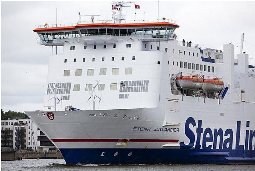
Figure 74: VAWT placed in the front of the superstructure to reduce air resistance & for power generation.
