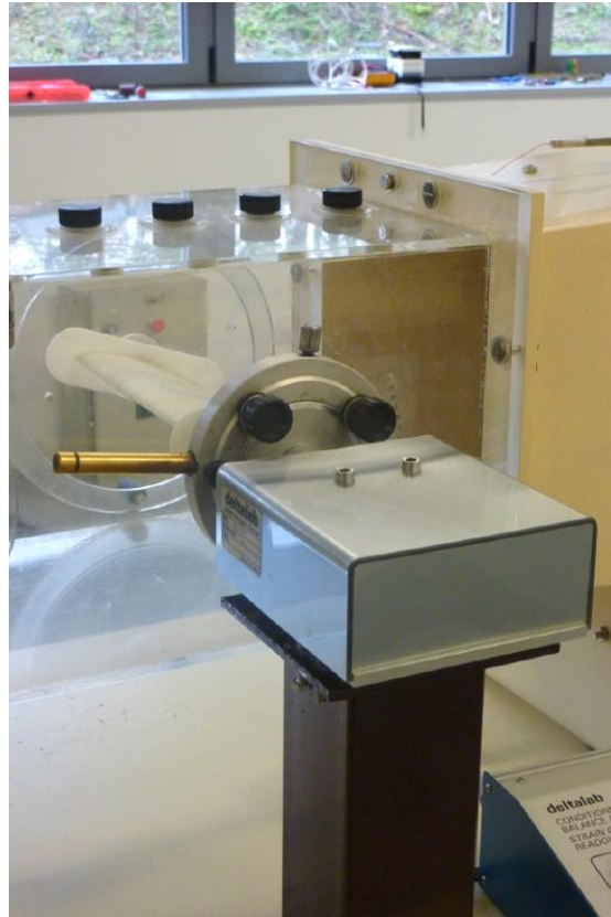
Figure 27: Load cell and foil blade arrangement.
