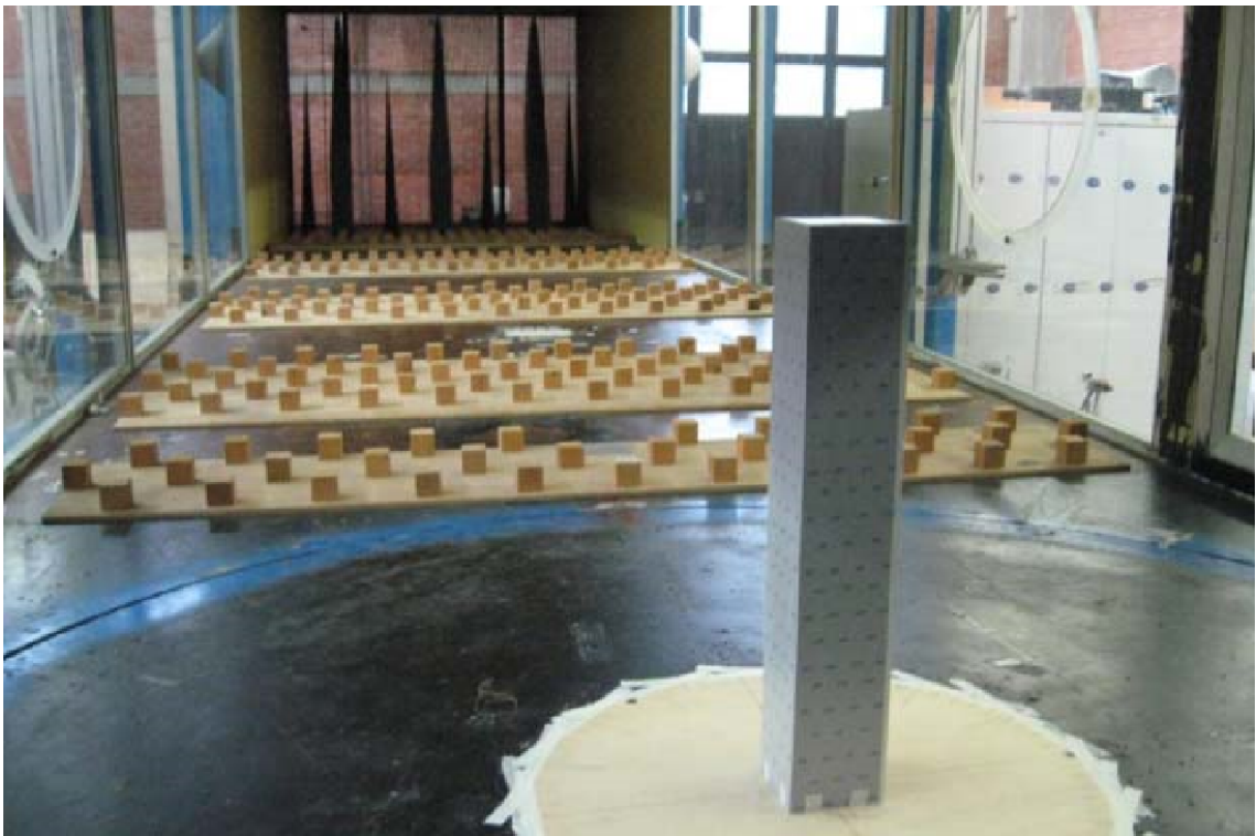
Figure 1.6: Example of ABL wind tunnel test.
