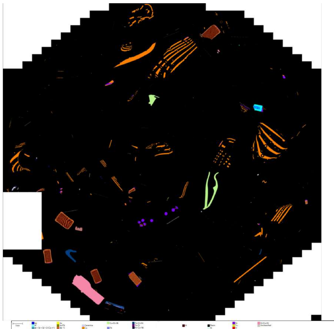
Figure 9.10: Full composition map of a section of crushed smartphone particles (II)
