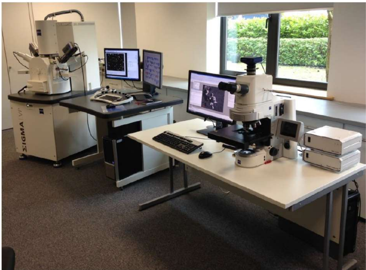
Figure 3.3: Image showing the Axio Imager. Z2M and the Mineralogic SIGMA VP at the ZEISS Natural Resources Laboratory, Cambridge.
