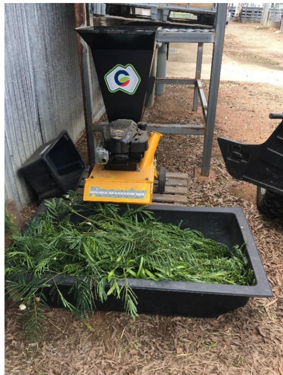
Garden chopper used to chop up the stripped edible material (Photo: Ed Charmley)
