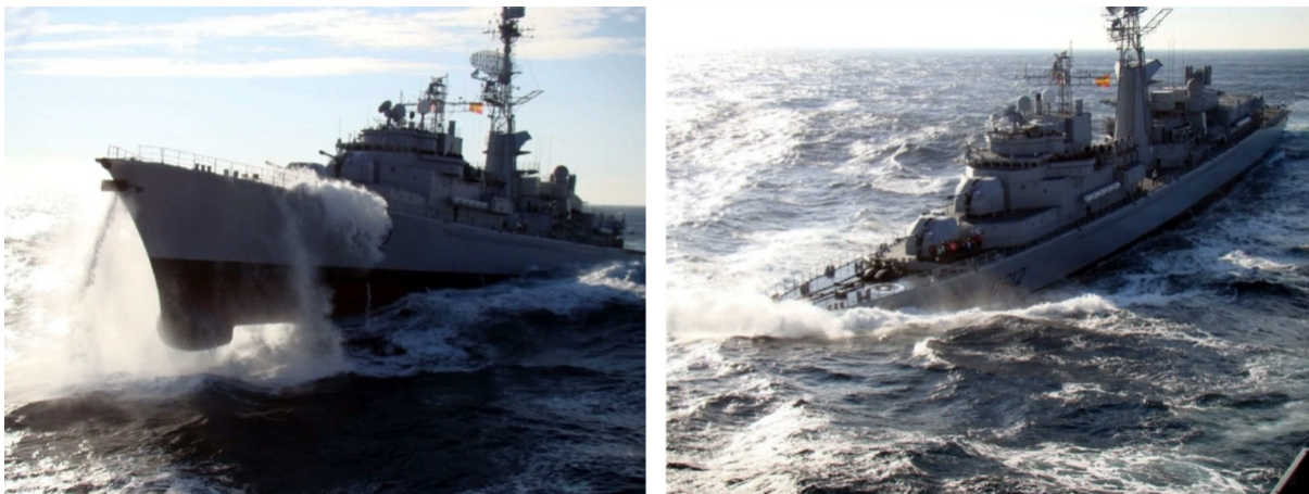
Figure 2: Slamming on the frigate De Grasse (From: Tassin, 2011 [6]).
