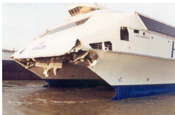
Figure 3: Damage caused by wet-deck slamming in the high-speed catamaran HSS 1500 Stena (From: Lavroff et al., 2010 [35]).
