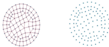
Figure 17: Comparison of FEM (left) and SPH (right) meshes (From: Messahel and Souli, 2013 [69]).
