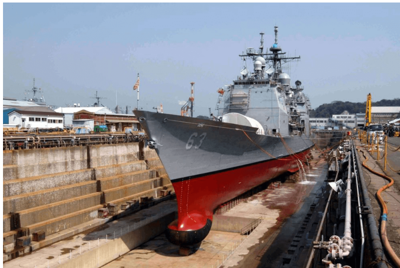
Figure 23: Port bow view of the USS Cowpens (CG 63) shows its sonar dome (From: [80]).
