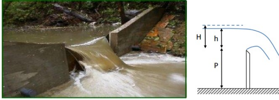
Figure 2.2: Flow over a sharp-crested weir
