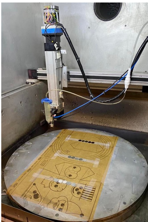
Figure 1.5: Set-up for the spray-coating process.
