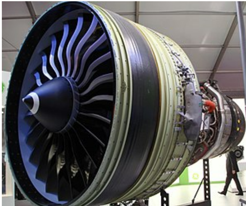
Figure 2.2: Engine GE90-115B soft-wall fan containment system [6]. It is composed by an inner metallic ring wrapped in Kevlar layers.
