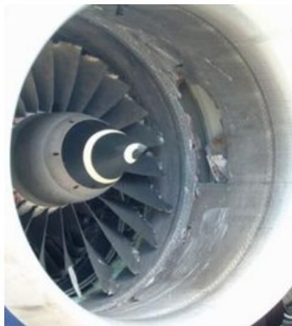
Figure 1.2: Damaged engine fan case from blade-off testing [39].
